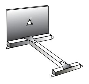
4. Cut a small triangular hole, to take the end of an inflated balloon, in a square of correx. Glue the correx to the frame.
