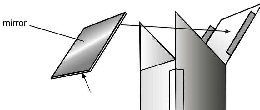
5. Fix A and B to the supporting flaps so that they are at 45° to the body of the periscope.
